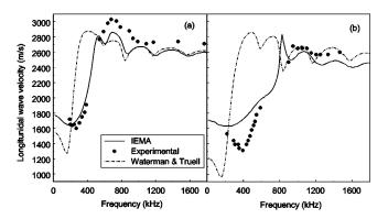
FIG. 5. A comparison between predicted and measured (Ref. 58) longitudinal velocity for a 660  $\mu$ m radius lead spheres in an epoxy composite with volume fraction (a) 26% and (b) 52%.
