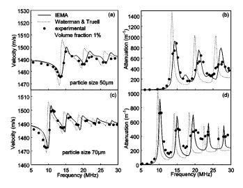
FIG. 8. A comparison between the predicted and measured (Ref. 16) sound velocity of a suspension of 1% polystyrene spheres in water with radius (a) 50  $\mu$ m and (c) 70  $\mu$ m and corresponding attenuation (b) and (d).
