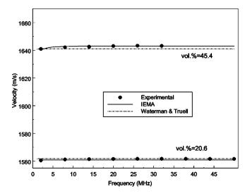
FIG. 10. A comparison between the predicted and measured (Ref. 15) sound velocity of a 308 nm polystyrene spheres in water suspension for different volume contents.
