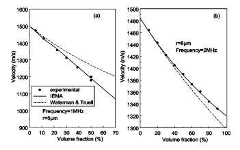
FIG. 13. A comparison between the predicted and measured (Ref. 18) sound velocity of (a) bromoform in water and (b) benzene in water emulsion.
