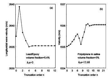
FIG. 3. (a) Velocity vs order *n* for 5.2% by volume composite of 660  $\mu$ m radius lead spheres in epoxy. (b) Velocity vs order *n* for 3% by volume suspension of 152  $\mu$ m radius polystyrene spheres in water.
