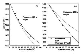
FIG. 14. A comparison between the predicted and measured (Ref. 18) sound velocity of benzene in water/40% glycerine and (b) carbon tetrachloride in water emulsion.
